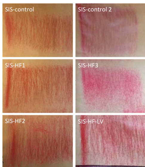
Fig. 3. Image of SIS adhesive spray pattern: optimized for solubility (left) and optimized for cost and low VOC (right).
